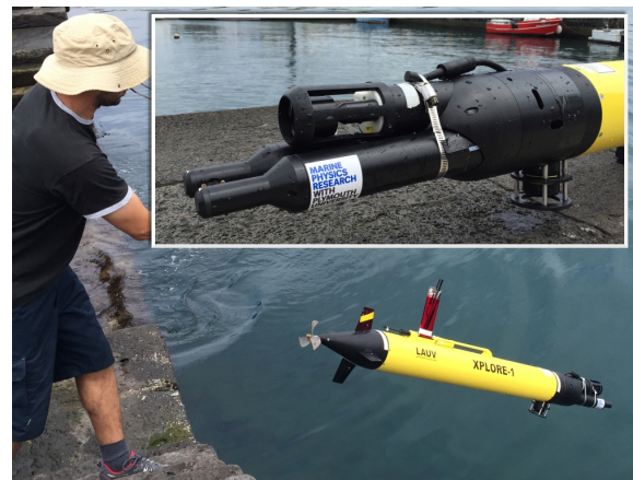
(a) Launching the LAUV-Xplore-1 off of a pier in the island of Horta for testing. Inset image shows the nose cone of the AUV with an experimental miniature holographic camera.
