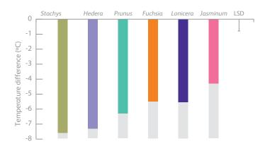
Figure 7.2: The extent to which different plant species can provide cooling to a building wall. The use of plant screens can reduce the amount of solar irradiance impacting on a building, thus reducing the requirement for artificial air conditioning. Comparison of a range of wall shrubs/ dimbers with *Stachys* as a comparison (Cameron et al. 2014).
