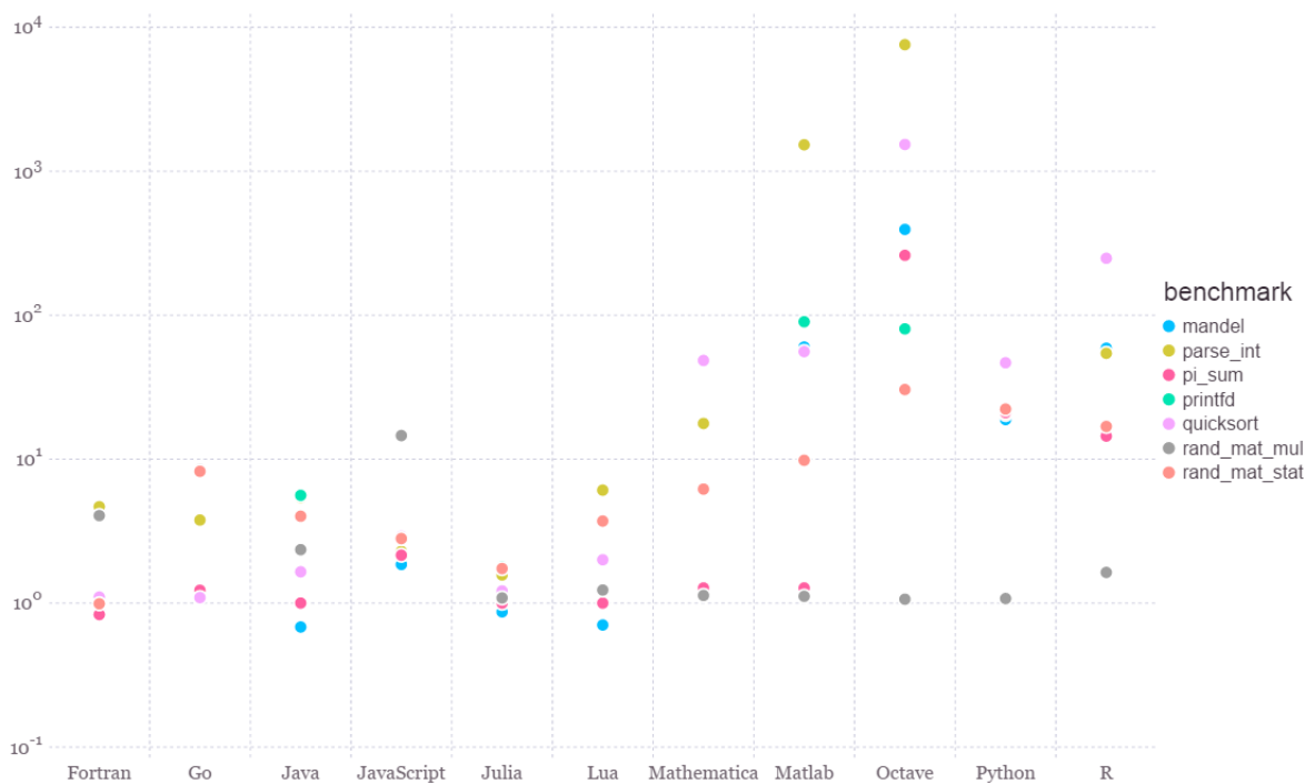
Figure 2: Smaller is better: the benchmark times for operations implemented in a number of programming languages relative to C
