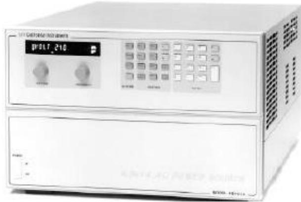
Figure 3.26: Picture of AC power source [12]
