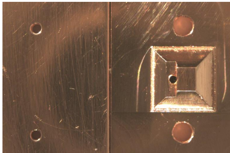
Figure 5.29: Zoomed view of surfaces that contact the die after polishing and cleaning
