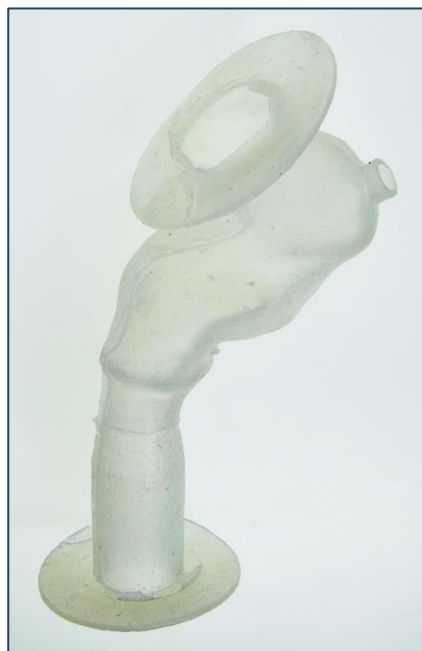
Figure 3.20 Image of the fabricated silicone rectum with casting runners removed.
