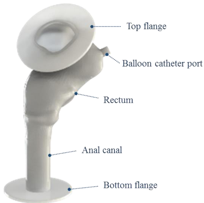
Figure 3.11 SolidWorks render of the 3DirCAD rectum model cast using the die mould, detailing its features.
