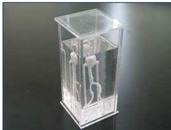
Figure 2.15 Physical model of the human cerebral artery fabricated from polyurethane and silicone elastomers. [135]
