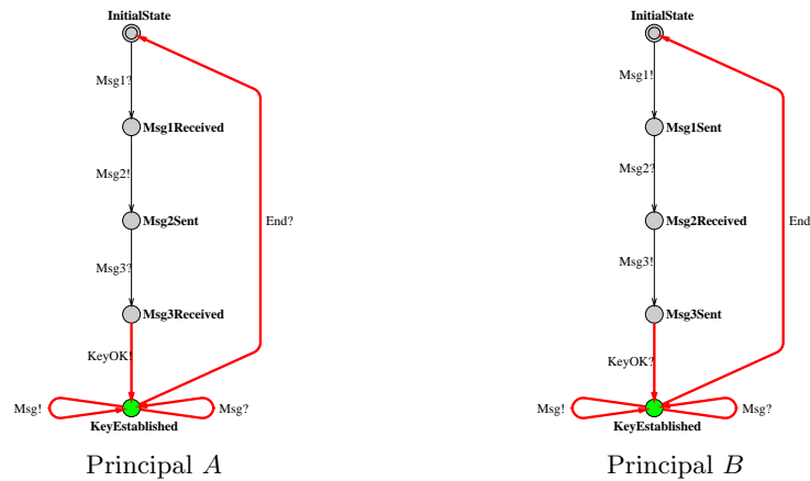
Figure 3. Extended BKE state-transition diagram
