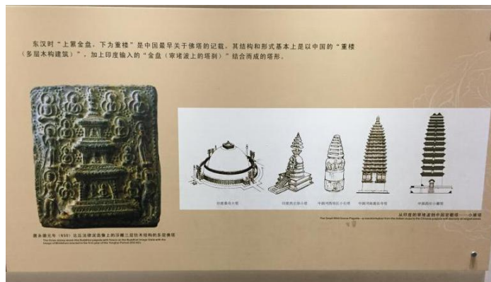
Figure 3.26 A diagram showing the correlation between Indian stupa and Chinese dense-eave pagoda.
