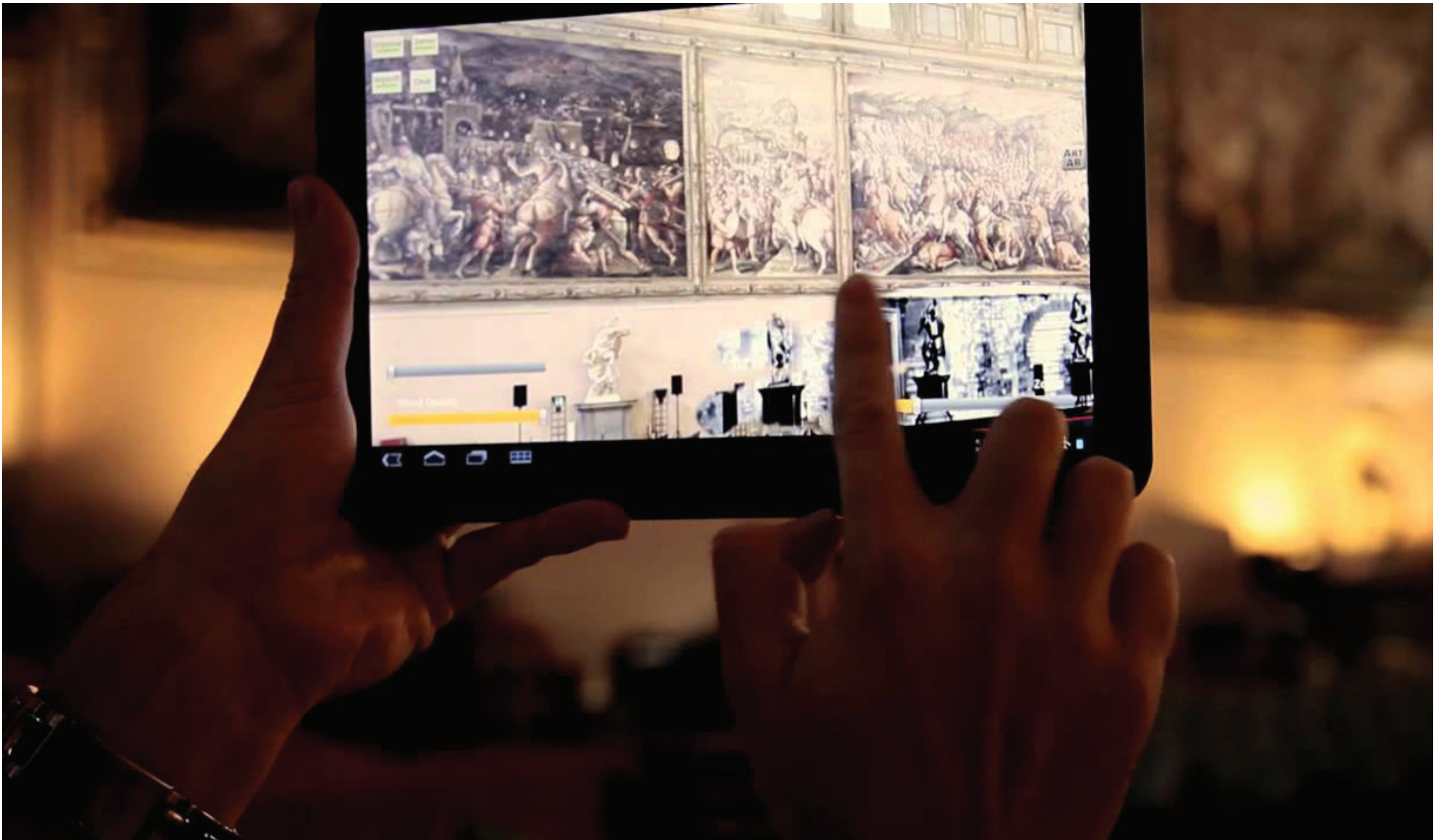
ARtifact user wipes away existing context to reveal x-ray data. Image: David Vanoni et. al.
