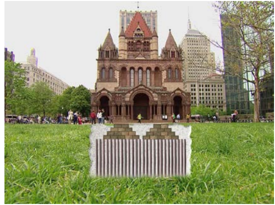
Fig 20. Trinity Church exterior animation of granite footing and wood piles driven into ground.
