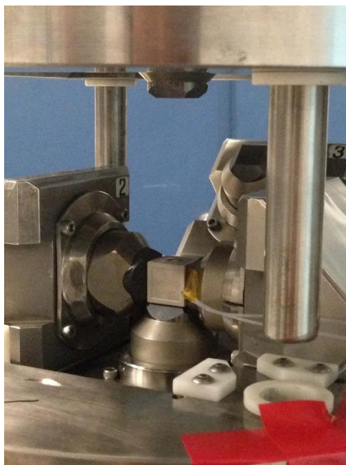
Figure 56. Schematic of the cubic sample cell assembly. Both the cube and the inner plugs are made of PEEK.
