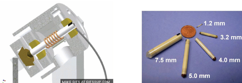
Figure 1.5 The scheme picture of the magic angle spinning module is shown. The right panel shows the Varian rotors with various diameters. The figures are taken from https://www.youtube.com/watch?v=13NLti-1ErA .
