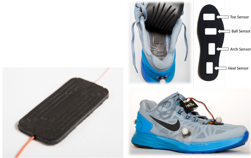
Figure 4.2: In-shoe sensor: (Left) NCPF sensor with wires embedded to measure the voltage response during impacts. (Right) Shoe equipped with NCPF foam sensors, microcontroller, and battery. The sensors were embedded under the insole at the heel, arch, ball, and toe.
