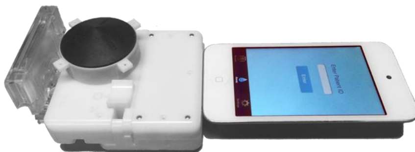
Figure 27. Image of smartphone dongle with a microfluidic chip connected to an iPod Touch (4 th Gen).
