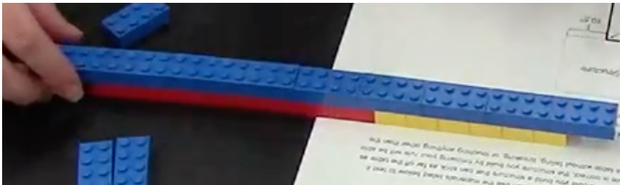
Figure 13. Build 1 cantilever for the low transfer pair. The front of the cantilever is considered the part on the left, which is lined with red Legos on the bottom. The back of the cantilever is considered the part on the right, with yellow Legos on the bottom.
