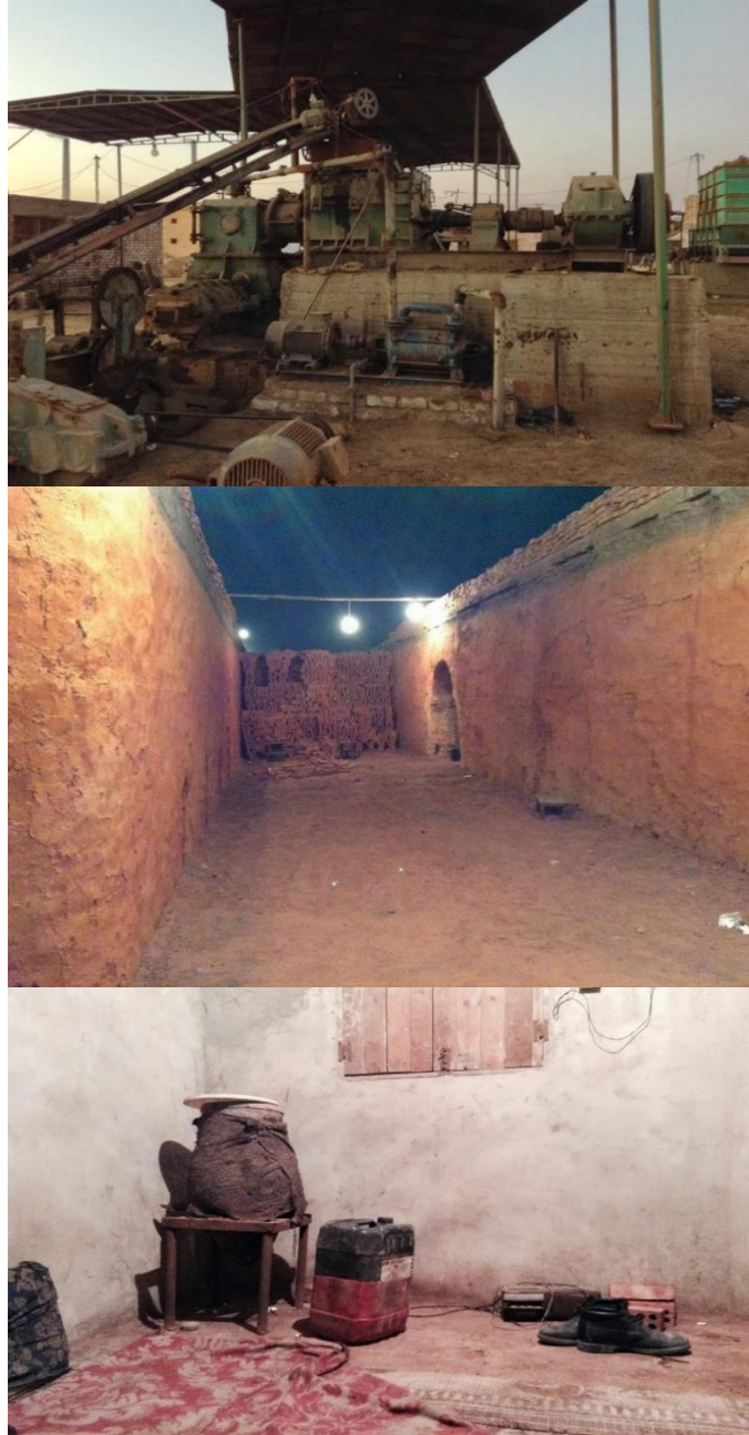
Figure 12: Part of the production line at a small factory maintained by Reda. The second picture is of the inside of the large oven (kiln). The bricks are stacked and the covered. The hareeq (burner) and his assistant then walk across a roof carrying between them a heat source that raises the internal temperature of the pictured space to over 900 degrees Celsius (1652 Fahrenheit). The third picture is of small resting room that sits atop of the kiln where the hareeq and his assistant rest between operations of their night long work. The hareeq and his assistant are separate from the rest of the workforce; often working when others are not and performing a task with a unique skillset and unique dangers. All photographs taken in an ad-hoc fashion on smartphone (Samsung Galaxy Nexus).
