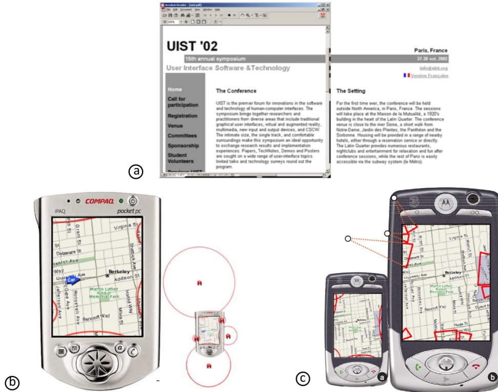
Figure 3.4: Examples of cue-based techniques. (a) City Lights [Mackinlay et al. 2003]. (b) Halo [Baudisch and Rosenholtz 2003]. (c) Wedge [Gustafson et al. 2008].
