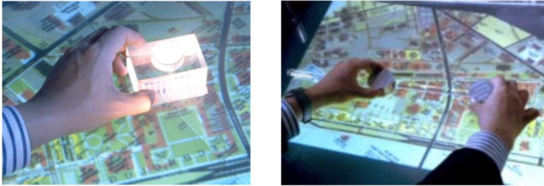
Figure 3.7: In MetaDesk [Ullmer and Ishii 1997], physical props are used to manipulate a map.
