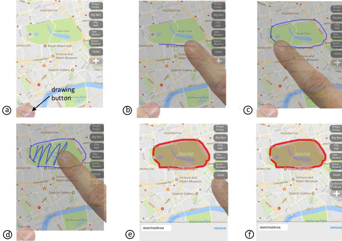
Figure 6.3: Drawing interface to mark custom spatial entities. (a) Holding the drawing button at the bottom left corner of the display, the user can then (b) sketch a line to specify a path or (c–e) sketch a (nearly) closed outline and scribble inside it to specify an area. (f) Tapping the “+” button at the lower right corner of the display creates a SpaceToken for the path or area.
