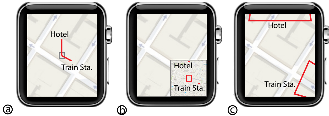
Figure 3.6: Where am I? Localization on a smartwatch form factor using (a) P-Compass, (b) Overview+Detail, and (c) Wedge. The two off-screen POIs are 6 cm (“Hotel”) and 4 cm (“Train Sta.”) from the centroid of the display. (In true scale.)
