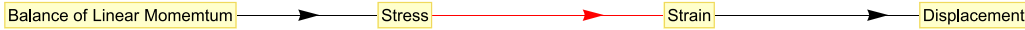
Fig. 1. Hierarchy of single-physics solid mechanics problem. Black arrow represents a definition or a “universal principle”; red arrow represents either a phenomenological relation or an operator that is defined not based on first principles. (For interpretation of the references to color in this figure legend, the reader is referred to the web version of this article.)
