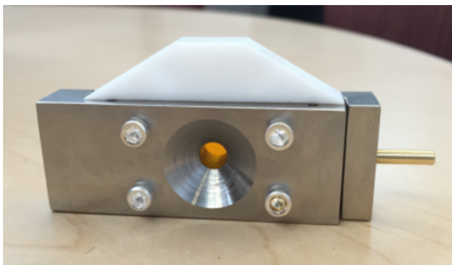
Figure 9.2: Static reaction cell. The pin on the right attaches to the goniometer to hold the cell in place. Precursor solutions are injected via syringe through the top ports, and x-rays penetrate the solution through the Kapton window in the center.
