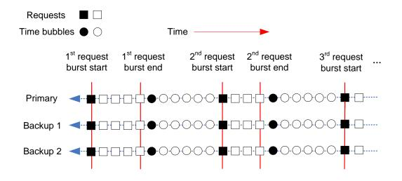
FIGURE 2.2: The request and time bubble flow.
