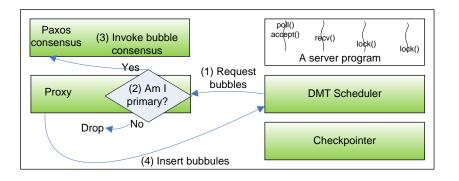
FIGURE 2.3: The work flow of inserting a time bubble.
