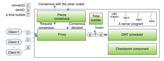
FIGURE 2.1: *The CRANE Architecture.* CRANE components are shaded (and in green).
