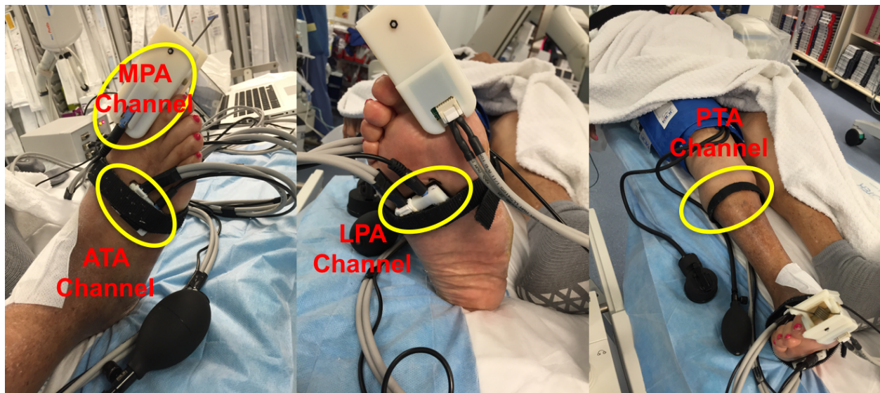
Figure 5.26 VOSM patch and toe clip placement on a PAD subject. Each channel monitors perfusion on an angiosome.
