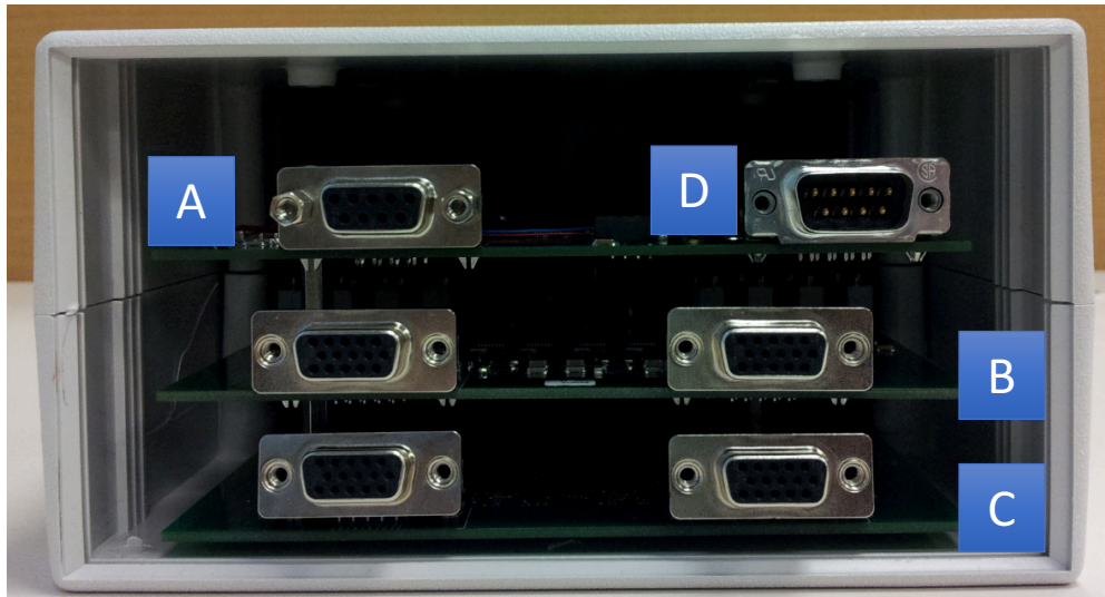
Figure 5.11 VOSM system enclosure with system electronics. There are three electronics boards in the enclosure, with the motherboard on top (A), and two acquisition boards below (B, C). In addition, there is an expansion connector to control a legacy optical switch (D).
