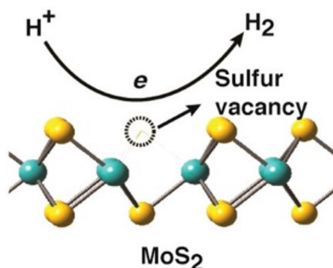
Figure 4.7: Schematic of the catalytic reduction of protons by the sulfur vacancies in MoS 2 . Figures reprinted with permission from reference 84. Copyright 2016 American Chemical Society.
