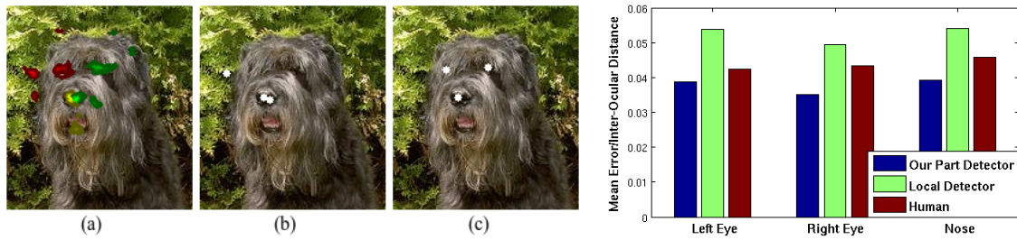
Figure 3.7: Left: An example of part detection. (a) Original image overlaid with heat maps from part detectors. Red is used for the left eye, green for the right eye, and yellow for the nose; better scores are shown as brighter. (b) Detected parts using the maximum value of the detection scores. (c) Detected parts using our full model. Right: Mean localization error divided by the inter-ocular distance.
