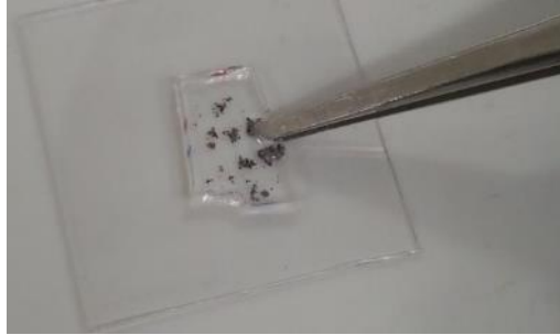
Figure B-5: Placing PDMS onto PETG on a hot plate.
