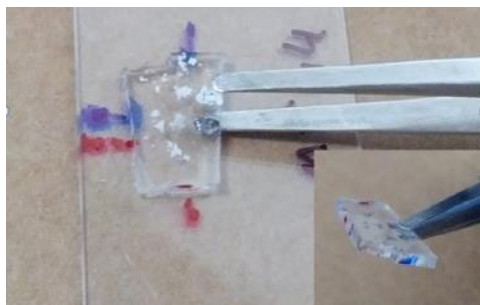
Figure B-4: Gently removing the PDMS from the slide. The bottom-right inset shows the marking on the PDMS after it has been lifted off.
