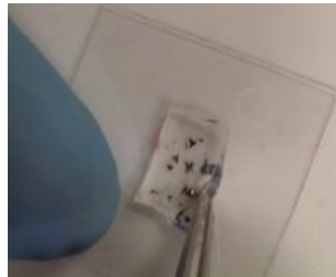
Figure B-6: Removing PDMS from PETG at normal incidence.
