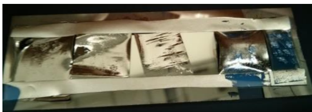
Figure B-2: Various tapes of \text{MoTe}_2 crystals coated with a layer of 100 nm Au.
