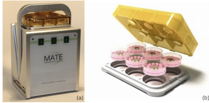
Figure 3.2: (a) Image of the MATE, assembled, and ready for culture in the incubator. A 6-sample tray (b) sits on top of the unit and voice coil motors drive each sample dish up into the polysulfone lid to create compress. Plastic guards surround the sample and create a guide for platens while keeping the sample safely underneath.
