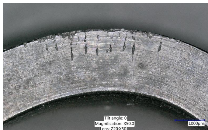
Figure 10 Multiple cracks found in an AISI 4140 U-bend sample LSP three times at 300 mJ. Unlike the stainless steel, the high strength steel fails by many parallel cracks rather than one major failure.
