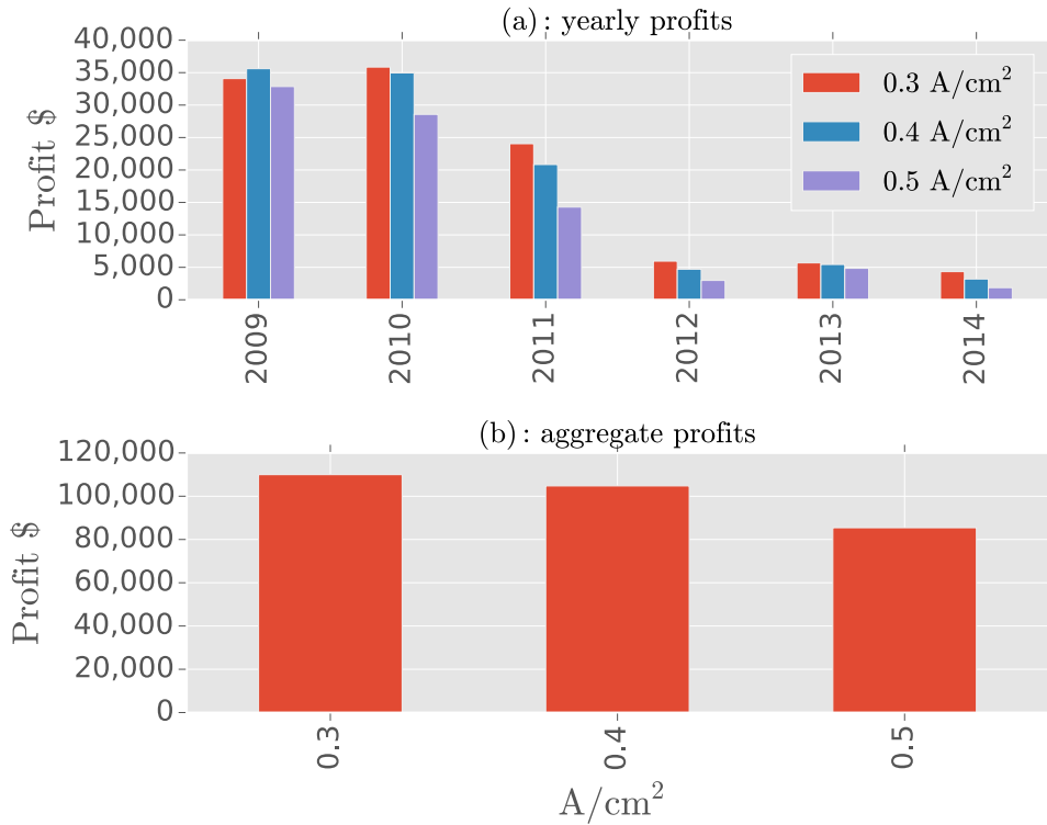
Figure 5.29: Fuel cell only: (a): yearly profits for different operating currents; (b): aggregate profits for different operating currents
