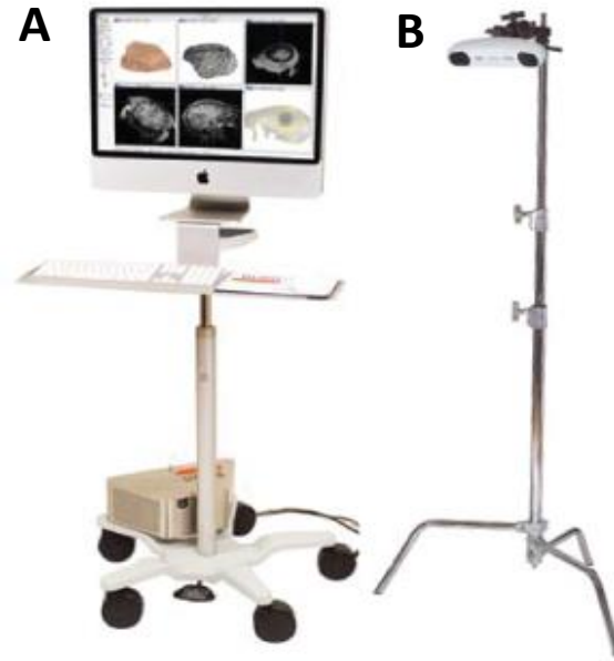
Figure 1.8. Neuronavigation system (Brainsight). (A) Computer to store and process brain images. (B) Position sensor camera.
