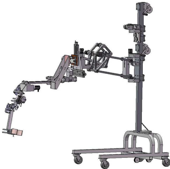
(a) A CAD model of the ALEX II exoskeleton.
