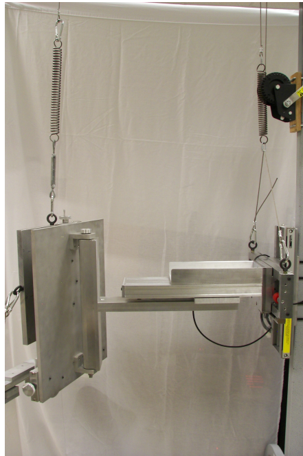
Figure 7.2: The initial support system for ALEX II, consisting of a series of prismatic joints.
