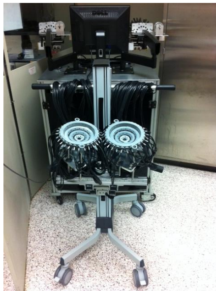
Figure 2.2 Image of the DOT breast imager with translating ring interface.
