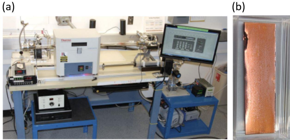
Figure 2.4. (a) CVD system used for graphene growth (courtesy of Hone's group) (b) Copper foil right after CVD synthesis.
