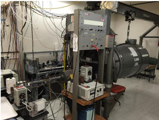
Figure 5.1. (a), (b) BNL's Van de Graaff used for the radiation of our devices. All e-beam tests conducted in ambient environment.
