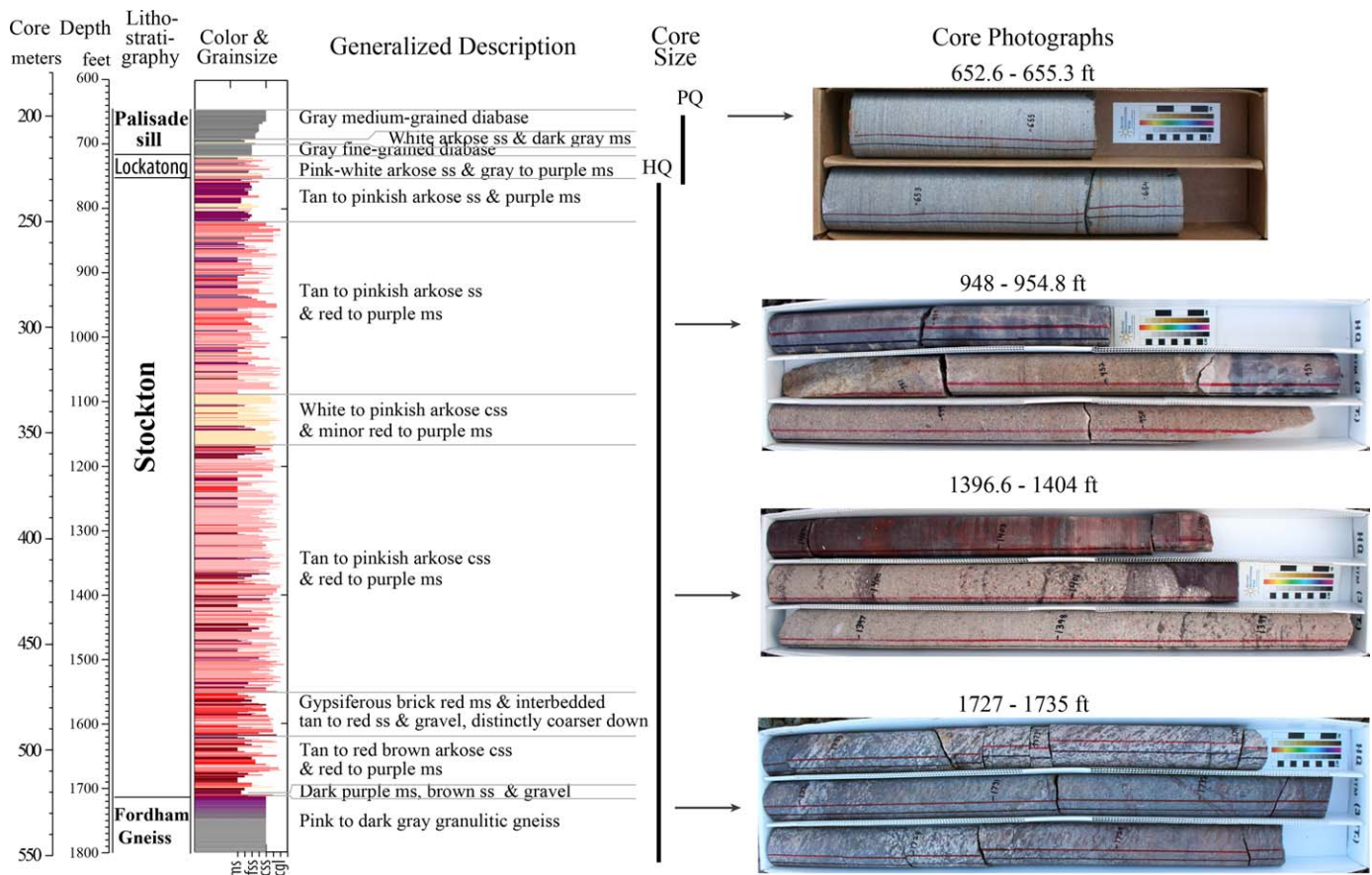
Figure 2. Lithological description of the TW4 core. From left to right: depth of the core, lithostratigraphic units, color and grain size of individual strata (ms—mudstone, fss—fine sandstone, css—coarse sandstone), core size, and photographic images of representative core intervals.
