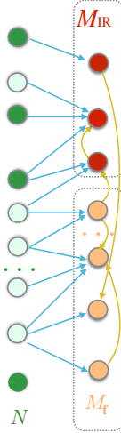
Figure 2.3: Illustration for the two subnetwork regime. The orange circles represent free units of the intermediate layer, all their feedforward inputs are silent for the given input patterns. They participate in the recurrent dynamics analyzed in section 2.4.4 The red circles denote input receiving units in the same layer.
