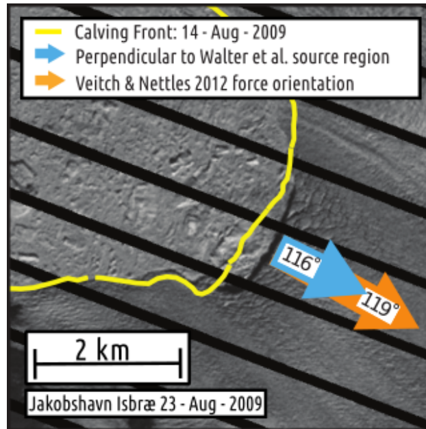
Figure 3.1: An example of a glacial earthquake with the source region identified by Walter et al. [2012a]. This image shows the calving front of Jakobshavn Isbræ after a seismogenic calving event, while the prior calving front is indicated in yellow. The angle perpendicular to the prior calving front is indicated by the blue arrow, while the force orientation as determined by Veitch and Nettles [2012] is indicated in orange. This image contains only the southern portion of Jakobshavn Isbræ discussed in this study.
