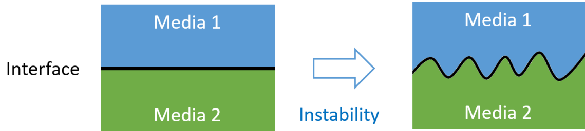
Figure 1.1 Instability at the interface between two mediae. Media 1 and 2 can be either fluid or solid.
