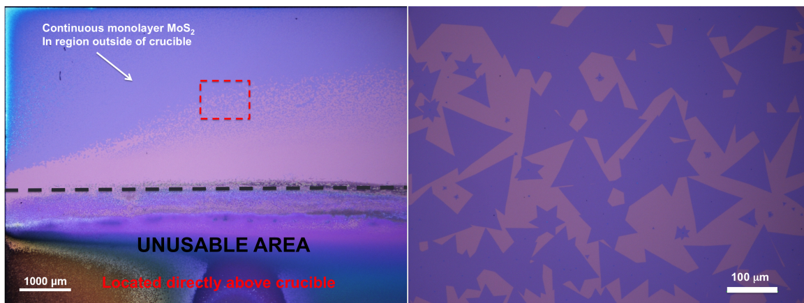
FIGURE 2.4. Optical images of growth substrate at low (left) and high (right) magnifications.
