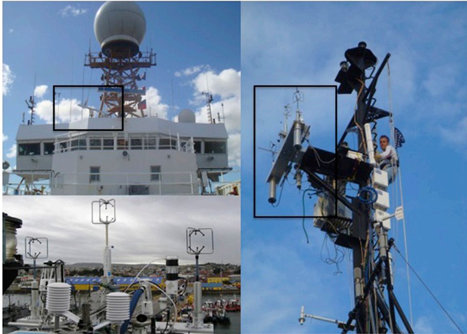
FIG. 1. (top left) The flying bridge of the R/V Ronald H. Brown , equipped with the Furuno 1510 radar (from the WaMoS system). (bottom left) The flux package, which contained all of the sensors that collected atmospheric measurements, was deployed on top of the mast (18 m above the mean sea surface). (right) The jack staff of the research vessel was outfitted with three sonic anemometers and two IMUs (black box).
