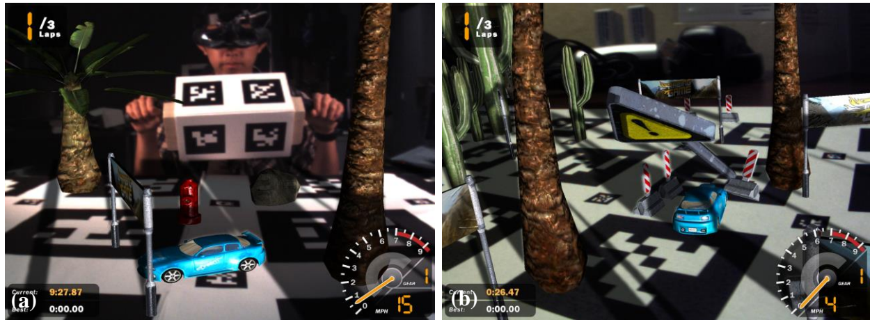
Figure A.13. AR racing game. (a) User holding an optically tracked controller and controlling virtual car on tracked physical gameboard. (b) Car collides with virtual signpost.
