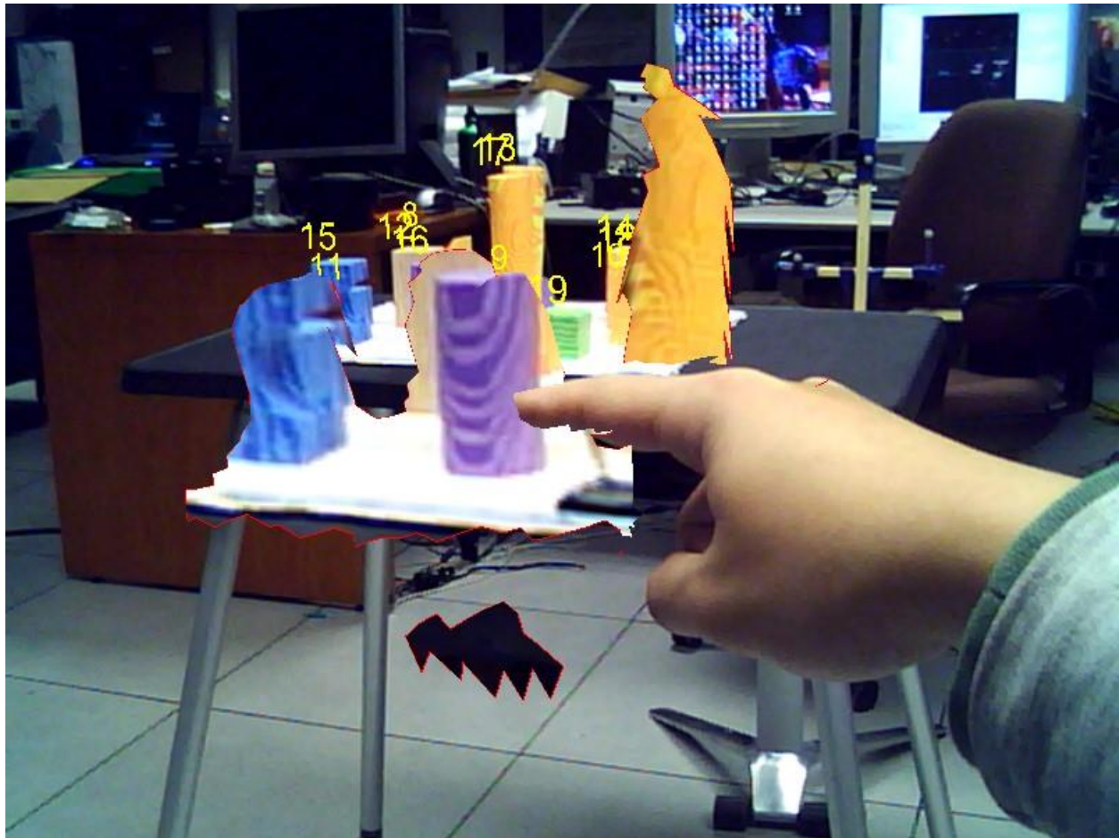
Figure 3.1. A selecting user (the indicator ) points at a close-up virtual representation of a portion of the physical environment sensed by a depth camera with her finger to indicate the target object. (The coarseness of the close-up representation and reconstructed virtual representation of the indicator's hand in this figure and the following figures is due to low depth-camera resolution.)
