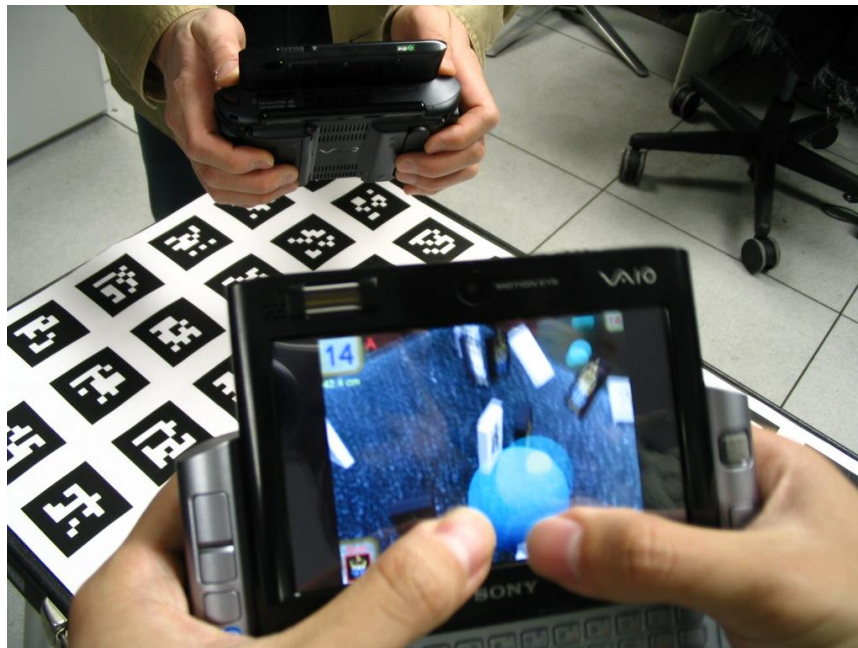
Figure 1.10. Player's view of our test application. Virtual balls are fired at virtual dominoes by tapping on the screen of a hand-held computer.
