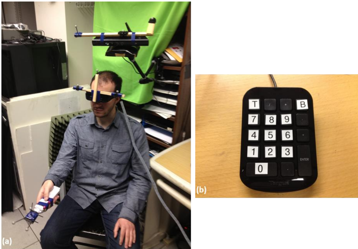
Figure 3.9. Hardware used for the techniques and the study. (a) The indicator, with tracked head-worn display, hand-held Wii remote, and Kinect mounted on shelf. (b) The numeric keypad used by the recipient.
