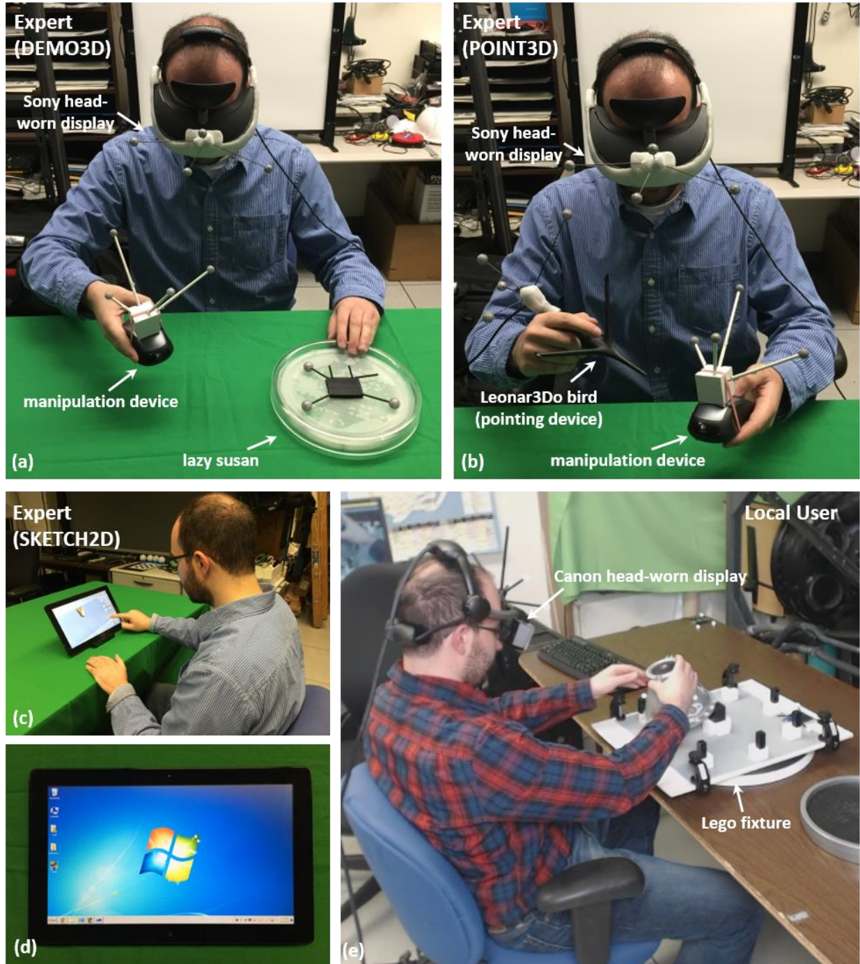
Figure 4.9. An expert wearing a tracked Sony HMZ-T3W head-worn display interacts with (a) a tracked mouse (manipulation device) and lazy susan turntable in DEMO3D, and (b) a tracked Leonar3Do bird controller (pointing device) and mouse in POINT3D. (c) In SKETCH2D, the expert interacts with (d) an untracked Samsung tablet. (e) A local user wearing a tracked Canon HM-A1 head-worn display places an aircraft engine combustion chamber top on a Lego fixture.
