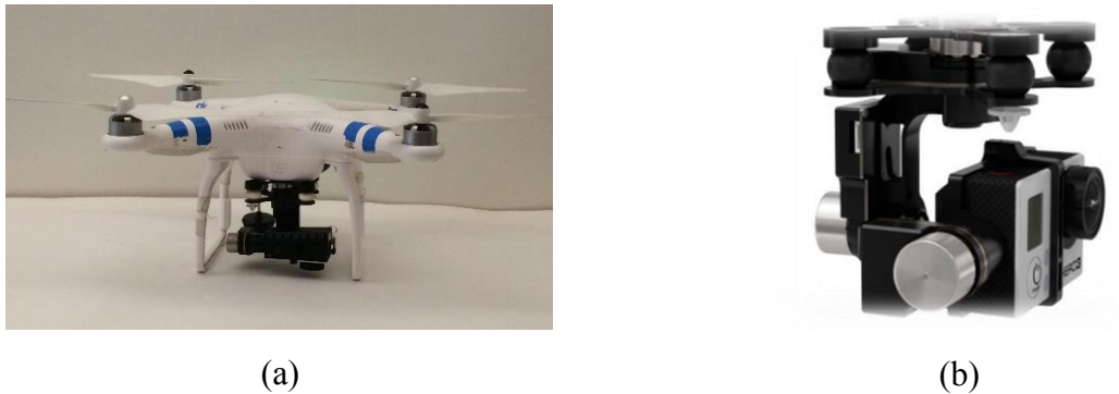
Fig. 0-1 The UAV traffic monitoring system used in this experiment: (a) the whole set-up and (b) the camera mount and camera
