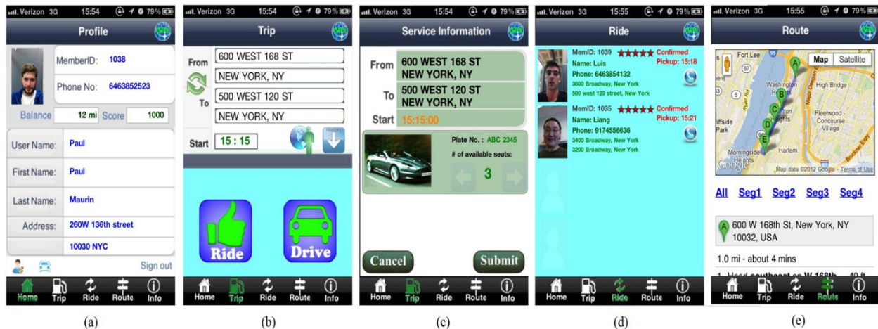
Fig. 0-6 Interface of the OMITS App on smart phones (a) member management, (b) new service request, (c) service information, (d) rider information for carpooling, and (e) dynamic route direction and pick-up sites
