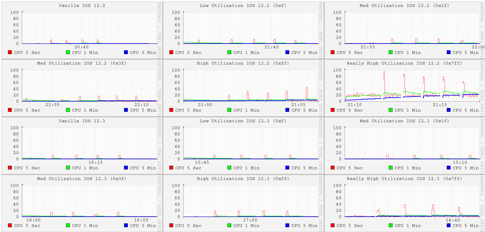
Figure D.1: CPU Utilization on Cisco 7121 Router Using Different SEM Payload Execution Bursts Rates ( g(\alpha_i, \tau_q) ) for IOS 12.2 and 12.3. Note the Direct Relationship Between g(\alpha_i, \tau_q) , SEM Payload Execution Time and Total CPU Utilization. Terms Low, Med, High, and Really High Utilization Corresponds to Varying SEM Payload Burst Rates, g(\alpha_i, \tau_q) .
