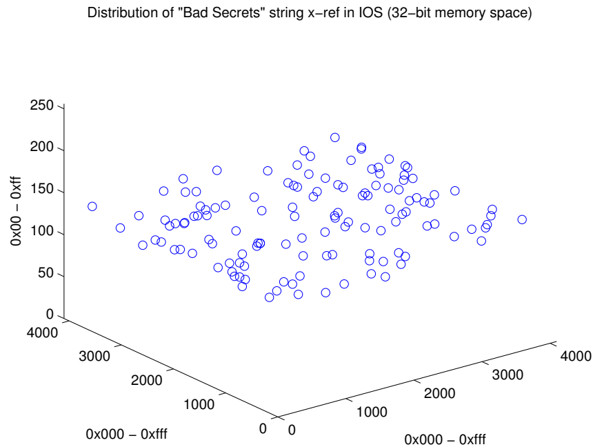
Figure 7.8: Distribution of the location of the password authentication function. This location varies greatly across the IOS .text segment, forcing the disassembling shellcode to search a large region.
