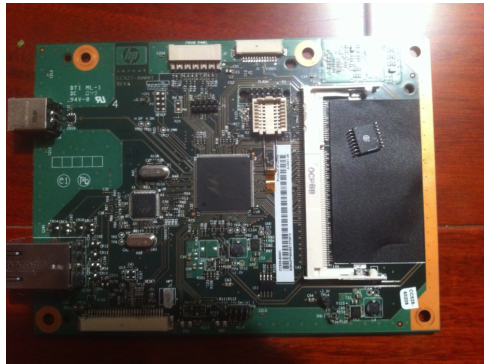
Figure 7.13: Formatter board for LaserJet P2055DN. Dump of the onboard SPI flash revealed RFU format and integrity checking algorithm.
