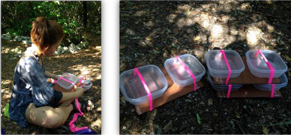
Figure 8. Diane assembling the containers to be placed at the bottom of the lagoons for sediment collection
