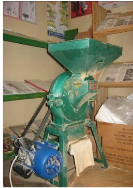
Figure 3: Vitagoat pressure cooker and stove in Bukura, Kenya. Figure 4: Soya Mill used to process soya flour and soya beverage purchased by CARD in July 2009
