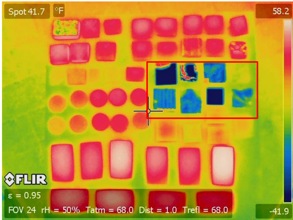
Figure 19: FLIR image demonstrating the variable range of metals shown in blue at cold temperature.
