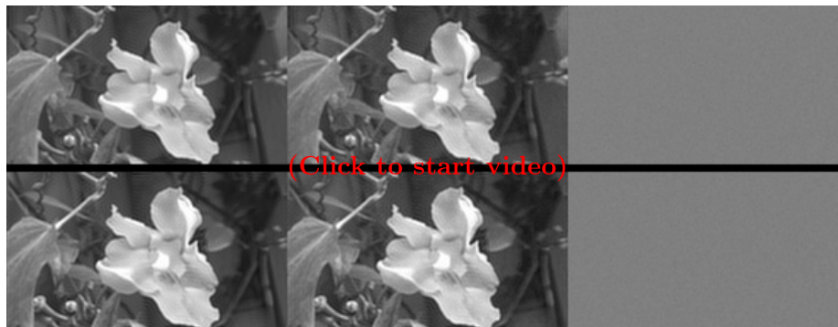
Figure 4.8: The original stereo video and the reconstructed stereo video in separate channels. The left eye channel is shown in the top row and the right eye channel in the bottom row. From left to right are respectively, the original video, reconstructed video and the error. (Modified from [118] with permission, ©2015 Elsevier)
