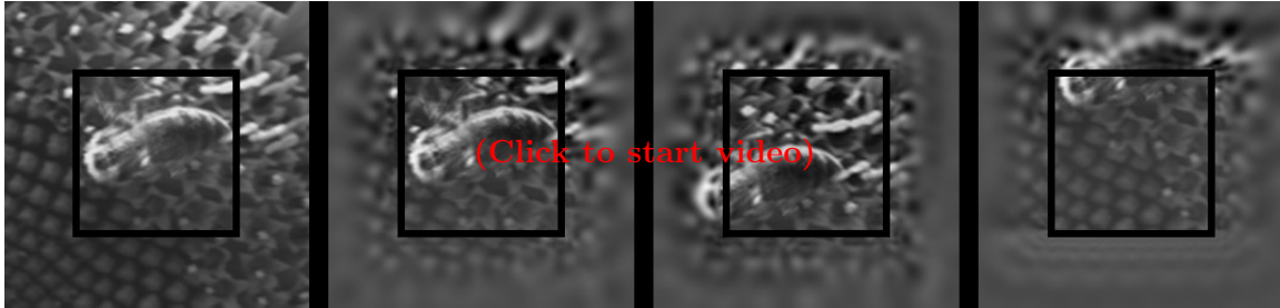
Figure 8.10: Translations of non-separable natural scenes on the Cartesian grid. The original video is shown in the 1st column. In the 2nd column, the original stimulus is recovered. In the 3rd column, the recovered video is translated downwards by 2 units and to the left by 2 units. In the 4th column, the recovered video is translated upwards by 4 units.
