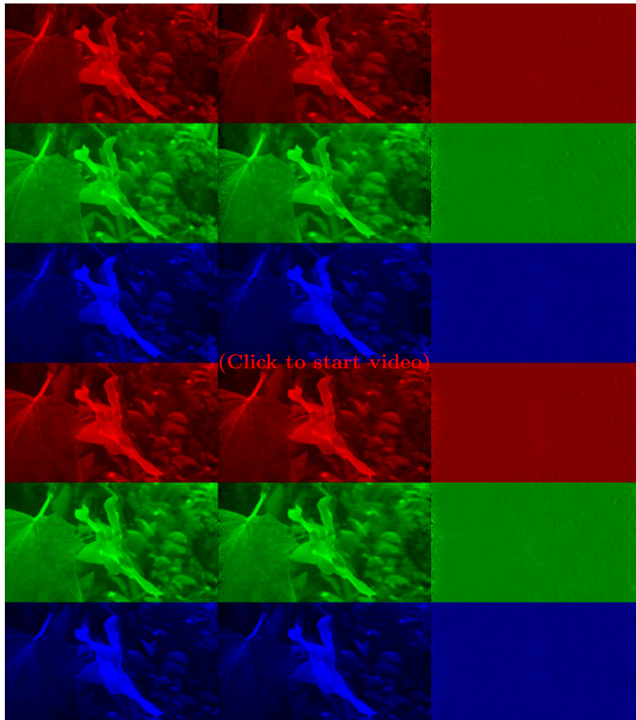
Figure 4.11: The original stereo color video and the reconstructed in separate channels. The first three rows are the color channels in the left eye and the last three rows are the color channels in the right eye. From left to right are respectively, the original video, reconstructed video and the error. (Modified from [118] with permission, ©2015 Elsevier)
