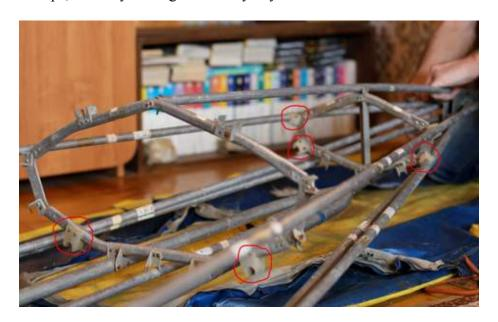
The duralumin carcass is lined with polystyrene foam (penoplast) – obtained from the Kirovsk
