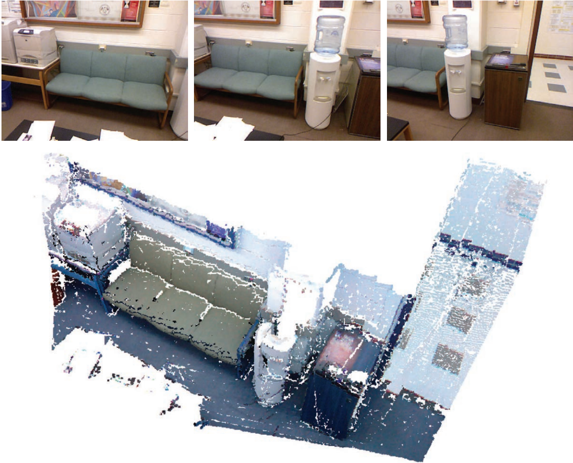
Figure 3.6: A sample scene of the Cornell Point Cloud Dataset used in our evaluation, including both the stitched point cloud and reference images.
