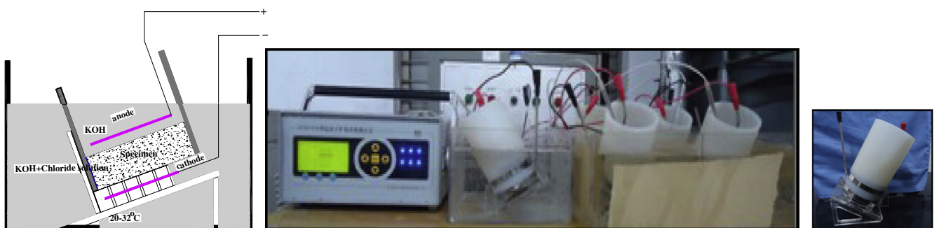
Fig. 2. Rapid chloride migration test setup used in this paper. (a) Schematic. (b) Actual. (c) Silica tube.
