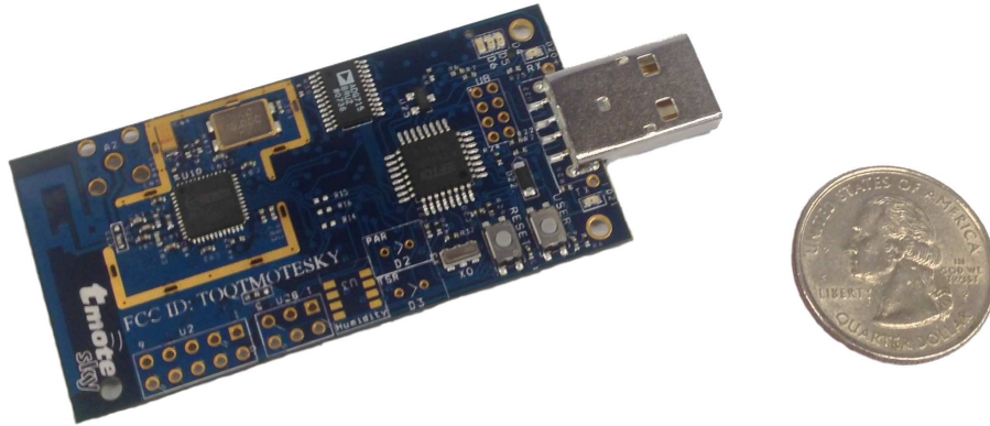
Figure 2.1: Tmote Sky also known as TelosB mote. This is the most popular mote used in WSN research and development. Most of the experiments presented in this dissertation were conducted with this WSN platform.
