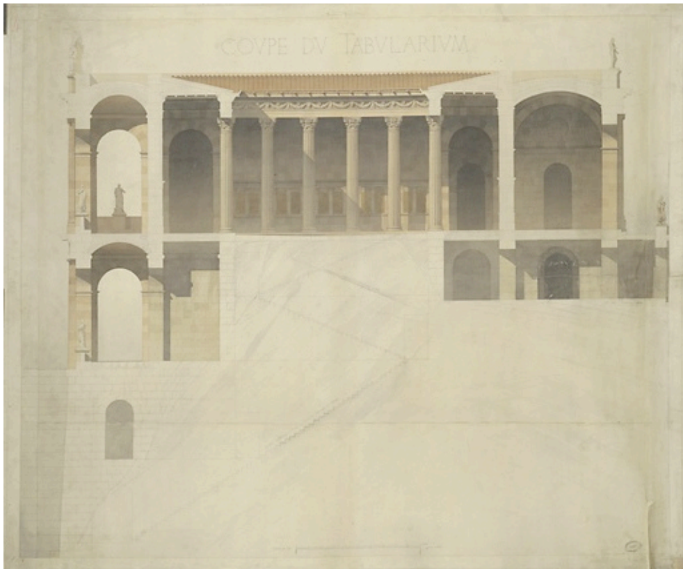
2.2.13 Constant Moyaux, (top) restoration of the Capitoline Hill with Tabularium in the background, (bottom) Section through the Tabularium showing the bronze tabulae adorning the interior portico, 1865. [École nationale supérieure des Beaux-Arts, Env 54-04]
