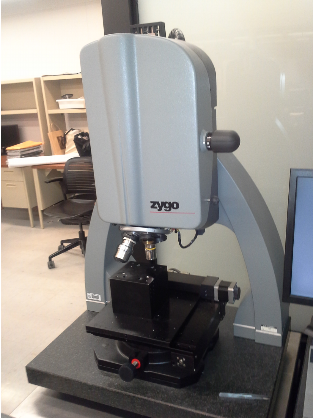
Figure J.8: Zygo Corporation, Metrology Solutions Division, 3D Optical Surface Profilers, Photograph # 2
