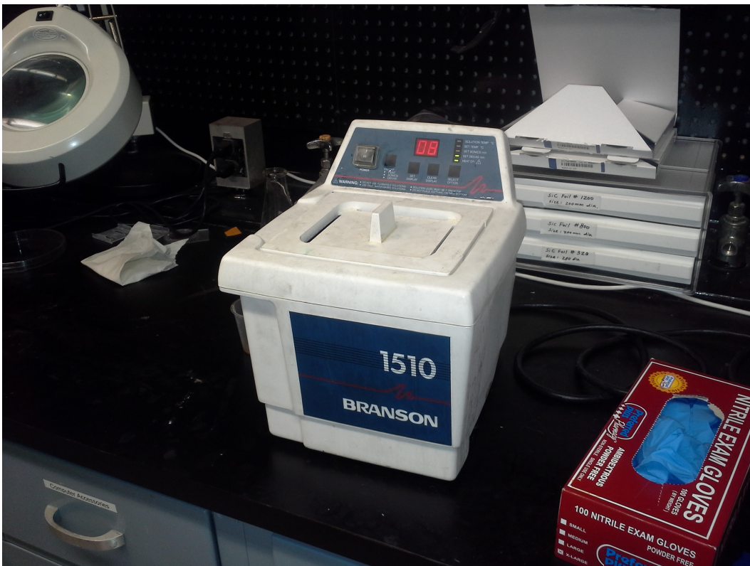
Figure J.6: Branson 1510 Ultrasonic Cleaner
