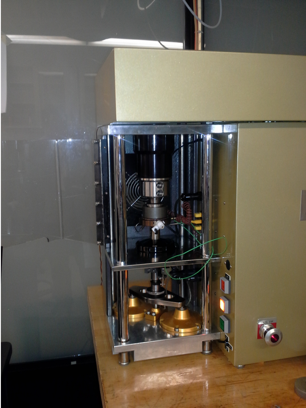
Figure J.4: Falex MultiSpecimen Test Machine, Photograph # 4
