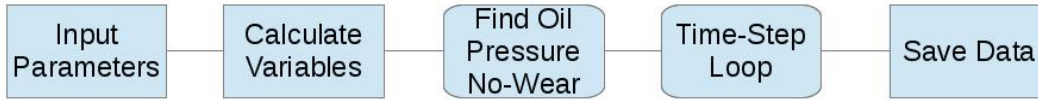
Figure E.1: Highest level flowchart of four-ball test wear model. The process takes place within the WearStudy.m script.
