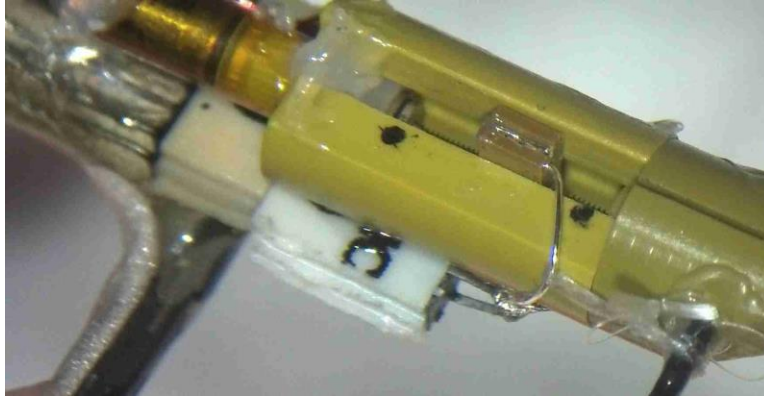
Figure A.6: Connect the electrode wire to the shuttle, glue it to the top of the shuttle, solder it to pin 14, and attach elastic string to the fixation bar and wire to add tension.
