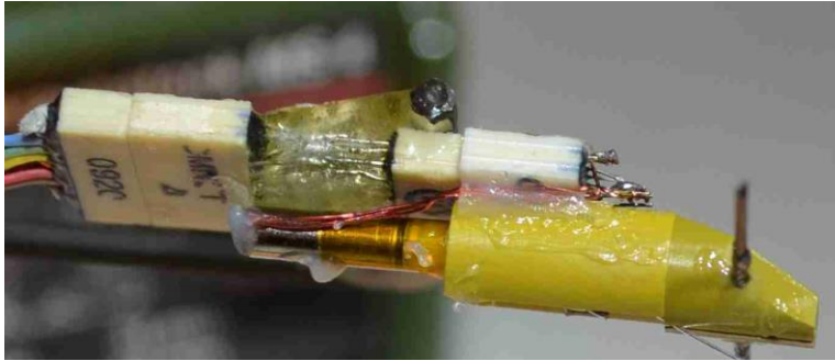
Figure A.5: Solder motor wires to pins 1, 8, and 9. Glue the wires into place along the junction of the body and omnetics connector. Insert a fixation bar (black pin) through the tip).
